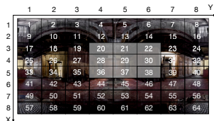
Figure: Illustration of tiles, viewpoints and FoVs in a 360 VR video. The grey area represents FoV 29 which is centered at viewpoint 29.
