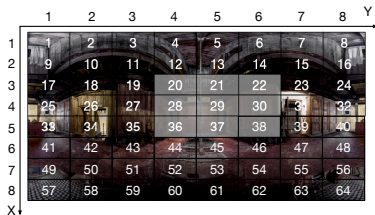
Fig. 2. Illustration of tiles, viewpoints and FoVs in a 360 video. The grey area represents FoV 29 which is centered at viewpoint 29.
